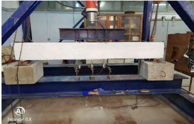
Fig. 9. Typical Beam during Testing.
