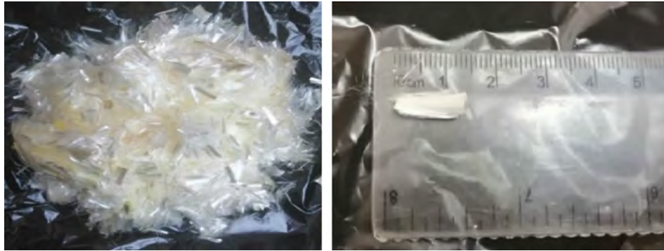
Fig. 5. Shape of Polyvinyl Alcohol Fibers (PVA).
